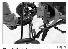
Step 4 Push down with your foot on therear lock brace until it is in the locked position. Fig. 4
