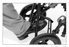
Fig. 15 **Step 5** up on center of brace with foot. **Fig. 15**
