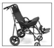
The anatomic back support frame stabilizes the neck and head in a functional position to assist the development of neck and head righting reflexes. The anatomic back frame is optional from the factory and must be ordered with the chair. Removable, reformable stiffeners are located inside the fabric seat back. Stiffeners easily pull out for custom forming with a heat gun. **Fig. 50**
