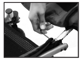
Fig. 48 Adjust seat depth to desired setting
