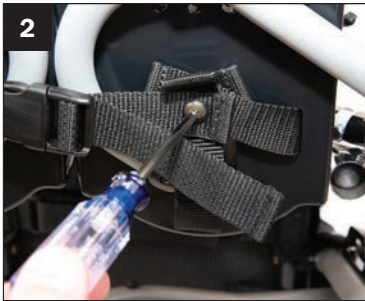
2. To remove the footplate securement strap, unscrew the screw on the bottom of the footplate using a screwdriver.
