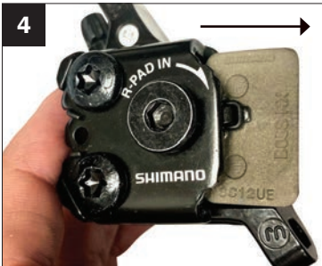
4. To remove pads, push pads through caliper.
