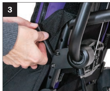
3. If required for additional height adjustment, unscrew the bolt holding the back positioner hardware onto the frame.
