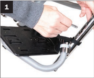
1. Pull on ring to remove detent pin holding footplate in place.
