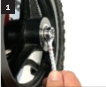
1. Loosen wheel with 5/8” wrench.
