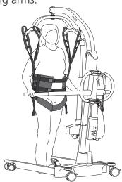
Lifter can be delivered with supporting arms, or complete lifting column with supporting arms can be delivered as an accessory to swap with original lifting column.
