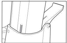
Fix the column by pushing the lock handle on the back all the way down.
