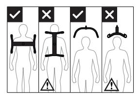
The sling bar must always be positioned across the user, to prevent the user from unintentionally sliding out of the sling.
