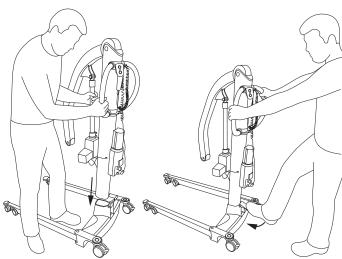
Place lifting column in chassis. Make sure that the red arrow on the lower part of the column corresponds with the edge of chassis. Make sure screw on column is inside the hole
