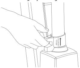
Pull handle on the actuator upwards to start emergency lowering, and the lifting arm moves downwards if under load. The lowering will increase in speed the higher the handle is pulled. Release the handle gently. Releasing the handle too quickly may cause person injury or damage to the lifter.
