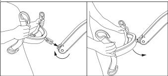
Insert bolt on sling bar in connection point to mount sling bar. When bolt is completely inside the sling bar is mounted and can rotate freely.
