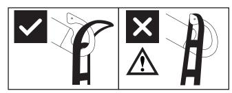
The sling bar's hook design prevents sling to be inadvertently detached when mounted correct.
