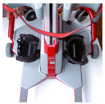
The sandals can be removed and replaced, only the hard side of the velcro will remain on the Molift Quick Raiser chassis.
