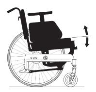
The front seat height is altered when the seat angle is adjusted. Starting from a flat seat:
