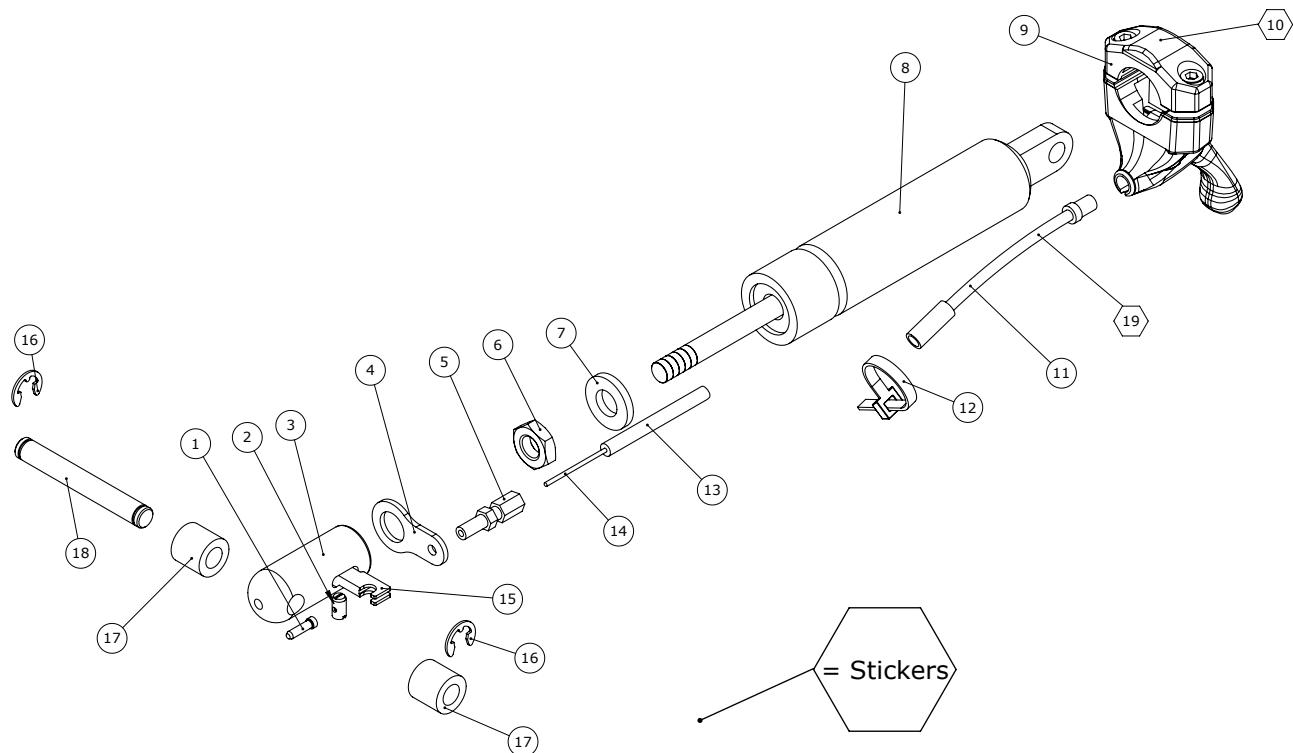
**Item numbers for Tilt lever kit for retrofitting on push brace, size 1-2 (163271, 95149)**
