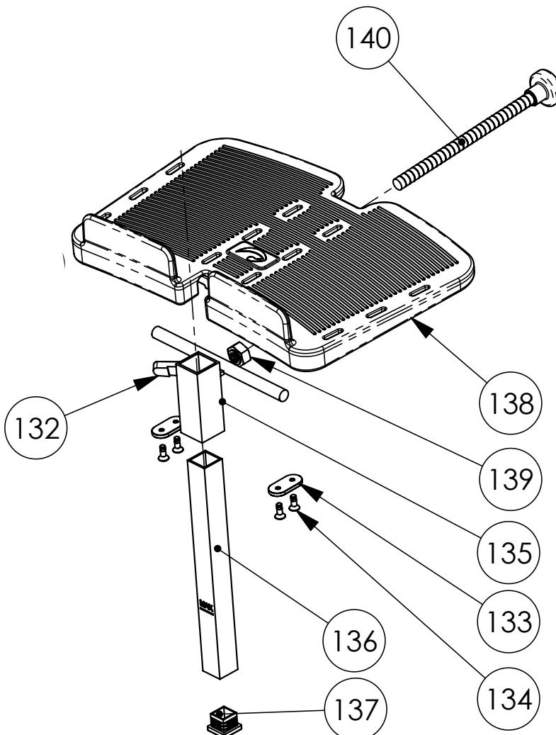
Item numbers for Foot plate without mounting fitting, Foot plate with 100 mm mounting fitting, size 2 (95145-1, 85145-2, 95145-2)
