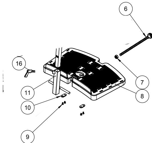
**Item numbers for Foot plate without mounting fitting, Foot plate with 100 mm mounting fitting, size 2 (95145-1, 85145-2, 95145-2)**
