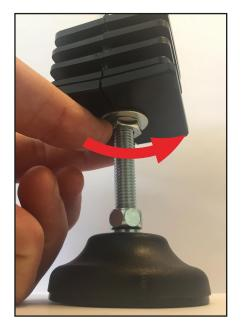
Turn the nut all the way up to fasten the plastic plug in the desired hight. Mount the levelling feet into the feet of the Molift Quattro
