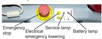
On the right side of the chassis there is a service light which will give a signal when the lifter needs service. When there is a green light, the lifter can be used normally. If there is no light, push one of the up/down buttons to activate the electronics, and the service lamp will illuminate. See the chapter "Maintenance".
