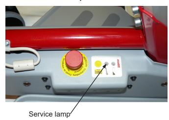
The electronics measures the operating time of the lifter, and after a specific time the service lamp will give a signal, first yellow light then red - indicating that the lifter needs service. Take contact with your local Molift service representative/dealer. The lifter can still be operated, but after a while an audible alarm will sound, to remind the operator that the lifter needs service immediately.
