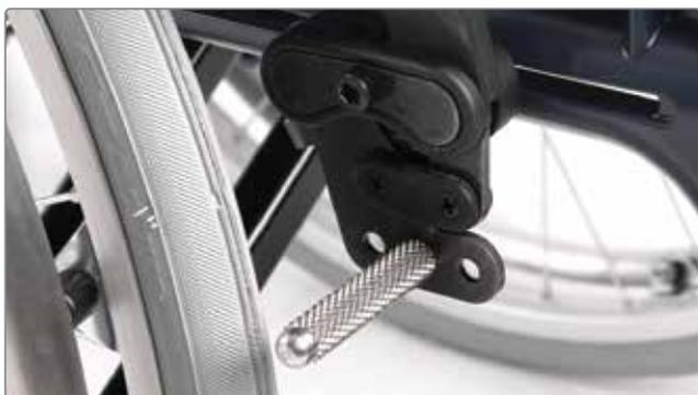
Distance should be 10-20 mm between tyre and brake. Always secure that brake applies properly, and that user can apply brake.
