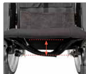
Gain an additional 0-7 cm seat depth by adjusting the strap back.
