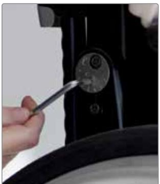
If the seat depth was extended in previous step, use allen key no. 5 to raise the lumbar support back up again. Unlock the screws indicated by lock symbol. Rotate by inserting the allen key in the small hole (marked with arrow). Tighten the locking screws now or after next step.
