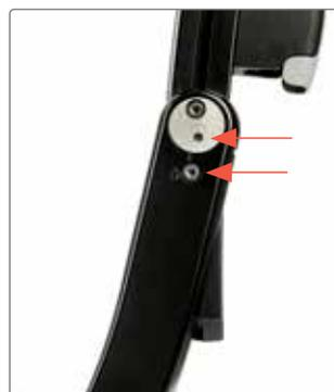
Loosen the locking screws with an allen key no.5. Slide the back height to the desired setting. 40 cm back height can often be a good starting point for the typical user (this will be fine-tuned at step 4.1).
