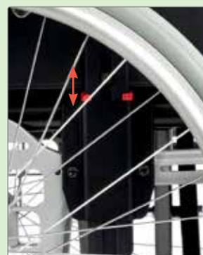
The arm support bracket can be moved vertically and horizontally.
