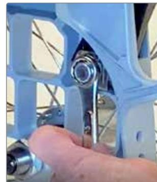
Prepare the seat depth by adjusting the hip angle using a spanner no. 13.
