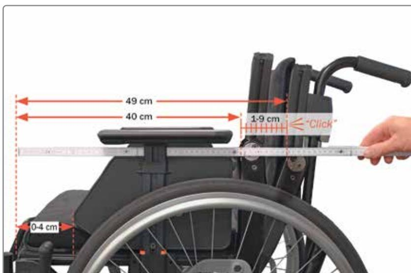
Standard frame: Seat depth is adjustable 40 - 49 cm in 9 steps, measured according to the picture.
