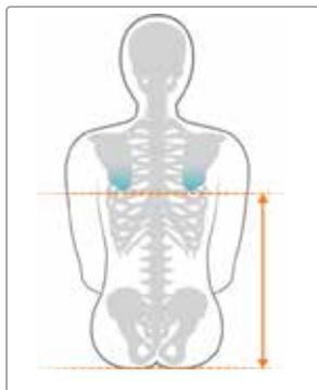
Adjust the back to the desired height according to users needs. Typical adjustment would be two fingers below scapula. See 4:3 below.
