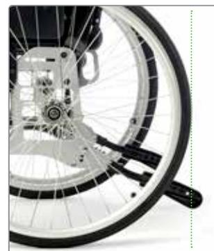
Distance for ground clearance should preferably not be less than 3 cm to climb small thresholds. Never place higher than 7 cm from ground.
