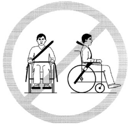
Figure 4: Belt restraints should not be held away from the body by wheelchair components or parts, such as the wheelchair armrests or wheels.
