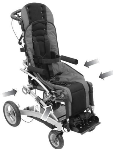
The optional wheelchair transport model has been crash tested and complies with the requirements of RESNA WC4:2012 Section 19 and ISO7176-19:2008.
